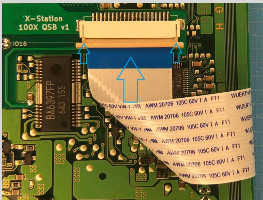
12. To ensure that the cable sits correctly route it through the slot on the top shield.
