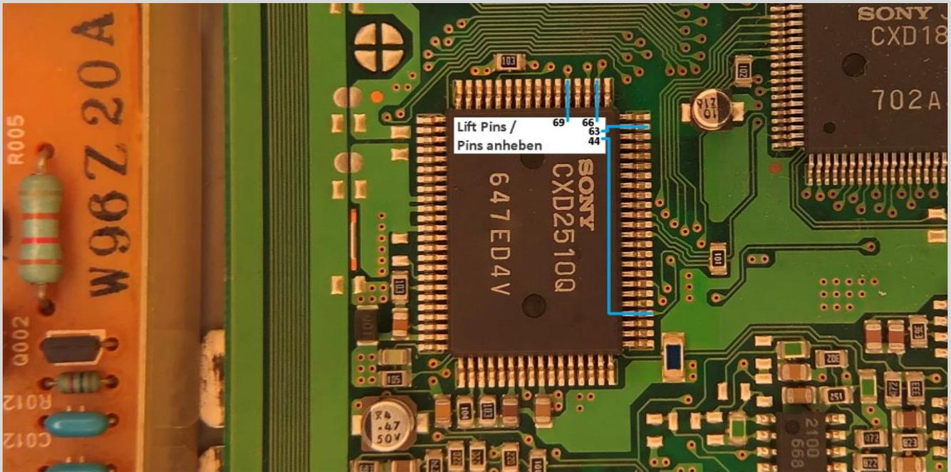
4. Please be careful not to damage the mainboard when lifting pins. Use a needle or x-acto knife and a fine soldering tip to simply touch the pin and apply some heat, then gently lift it from underneath using the needle or blade.
