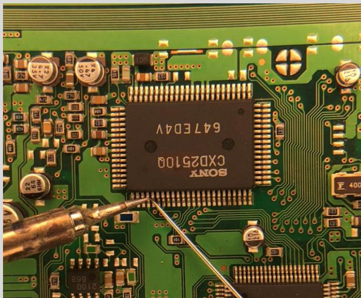
5. Please make sure that you have lifted the pins completely. They should not have contact with the motherboard, nor with each other.
