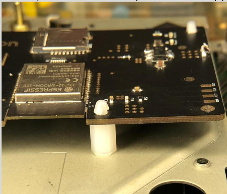
14. Now grab the other side from the flex cable and carefully connect it to the cable holder on the xStation. When it is done you have to fold the flexcable a bit. Folding it like this is best:
