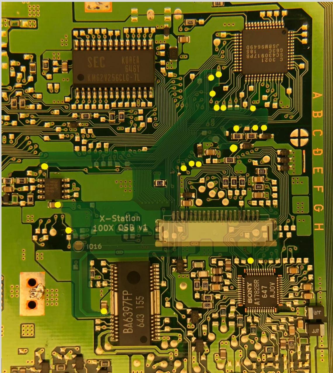
9. Connect the IO16 pad from the QSB to the marked location. Please ensure that the cable does not run over the metal areas where the shield could crush it.
