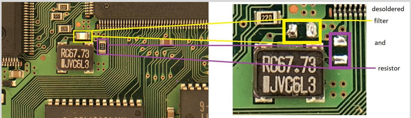
We are now finished with the top side of the mainboard; turn it bottom side up. Here, 3 resistors have to be desoldered and then the Quick Solder Board (QSB) installed.
