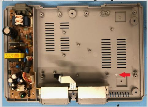
13. Now you have to connect the flex cable to the cable holder on the QSB. (blue side up) and close the cable holder. When this is done you can lead the flex cable outside
