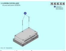
4. Remove the two long screws on the upper cabinet carefully
